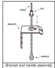
and a slight spring tension can be felt. Tighten brass lug with Allen wrench 1/2" above bracket (see
